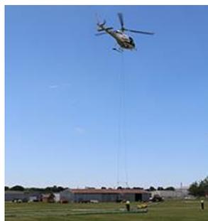
An aerial electromagnetic survey of the area was completed in the summer of 2016. The data gathered will provide the Lower Loup NRD with detailed information regarding overall depth and potential layering throughout the area's aquifer.
